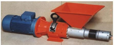
Figure 1. The mechanical oil press with special screw [Năsui 1997]
