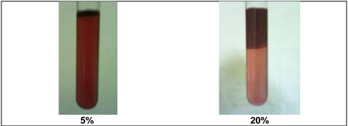
Figure 1: Separation of phases of winery waste. The dark phase is the surfactant rich phase.
