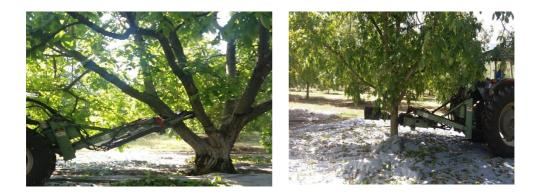
Figures 1 and 2. Mechanical harvesting of walnuts trees with a trunk vibrator accessory to a tractor of hydraulic type.
