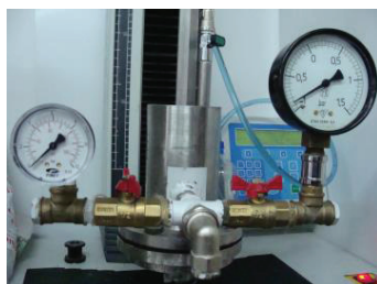
Figure 3. Experimental Equipment for pressuring cyclic and vacuuming cyclic process for meat tenderization (EE - PC.VC.P).
