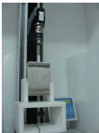
Figure 6. Universal testing machines Lloyd Instruments LRXPlus 5 and Warner - Bratzler experimental equipment
