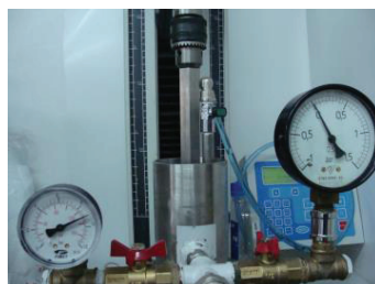
Figure 3. Experimental Equipment for pressuring cyclic and vacuuming cyclic process for meat tenderization (EE - PC.VC.P).
