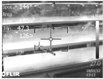
Figure 2. Thermovision scanning for closed oven heat losses up to 126°C
