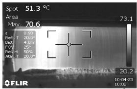
Figure 1. Roller mill overheating up to 73,1°C
