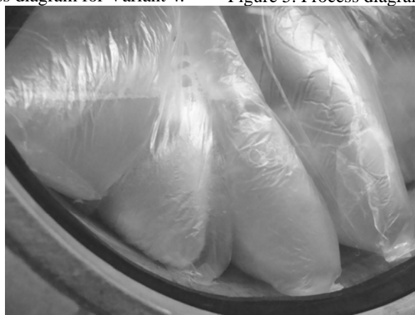
Figure 6. The vacuum infusion due to osmosis process during the vacuum evaporation in Variant 5.
