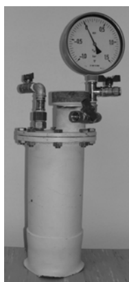
Figure 3. ZMS drying filter module for high corrosive gases
