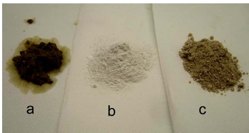
Figure 1. Olive OMW formulation; a: olive OMW mixed with talc powder 1:4 v:v; b: talc powder only and c: olive OMW mixed with talc powder 1:10 v:v
