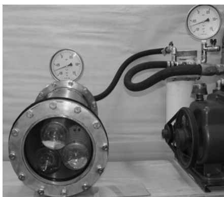
Figure 1. Experimental equipment for vacuum food processing
